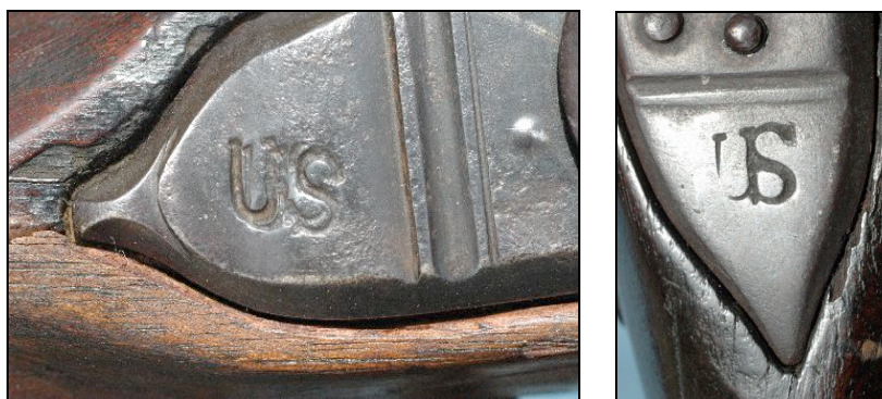
Locks of the Prahl and 1717 have similar conjoined US stamps with tailed U's that resemble the stamp on the breech of the Prahl, but all three are of different sizes. The US on the Prahl lock was double-struck due to problems with the case-hardened lock and the convex shoulder of the Germanic bevel; as a result, it appears disjointed.
