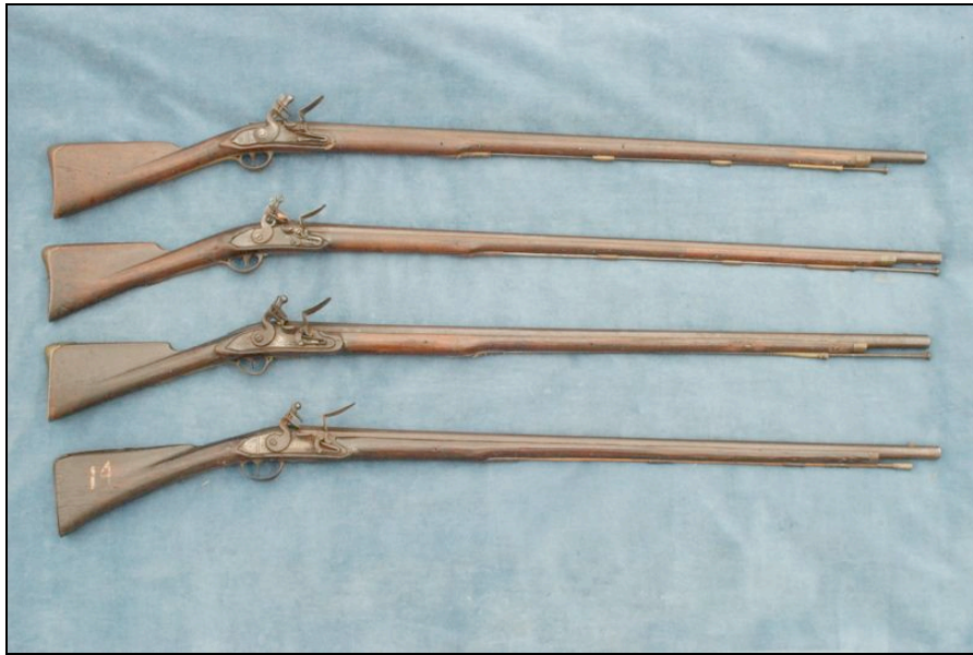
Four Philadelphia muskets, 1780-1783: three Continental-made and a M1717 rampart musket altered by Cowell (bottom). Top 3 in standard sequence for these photographs, derived from (top to bottom): Prah, M1766 Charleville, M1717 rampart musket.
