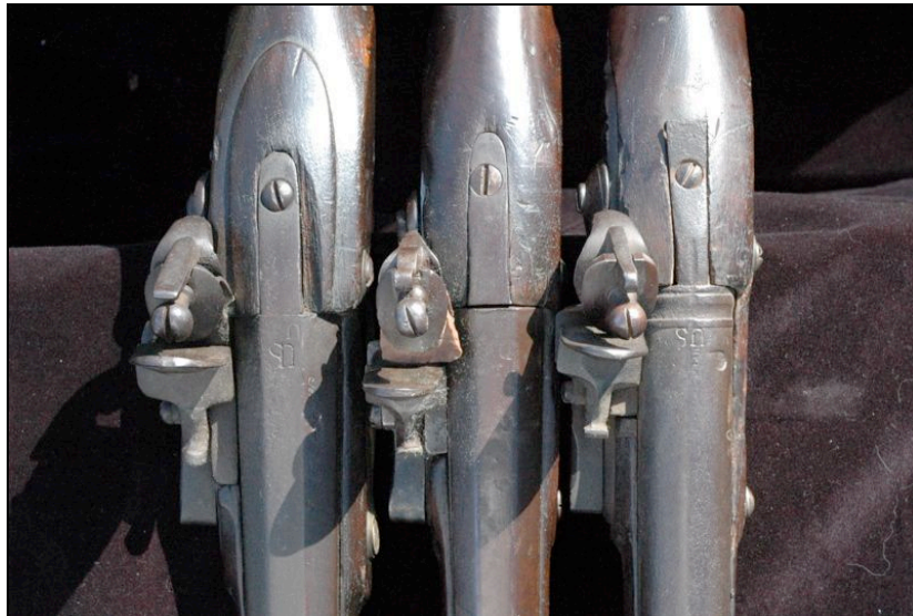
Though these Philadelphia stocks are in British style, only the M 1717-derived musket (L) uses the raised breech plateau of the antecedent British P1756. M1766 (C), “Prah,” (R).
